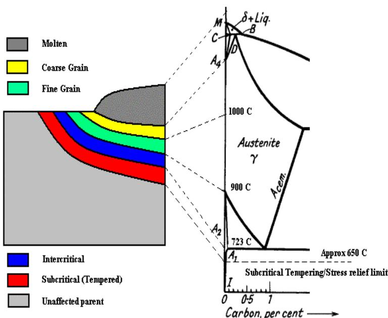
*Note: During welding there can be up to four sub-zones within the HAZ created according to the maximum temperature reached and the duration of time at that temperature.*
