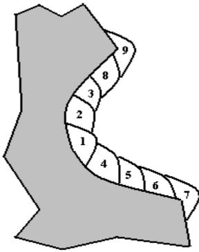
Welding Parameters 2.5 mm electrodes
